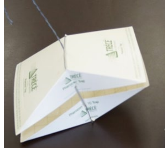
Picture 3. A wing trap used in a moth monitoring program. A pheromone lure is used to attract adult moths to the trap where they are captured with a sticky substance.
