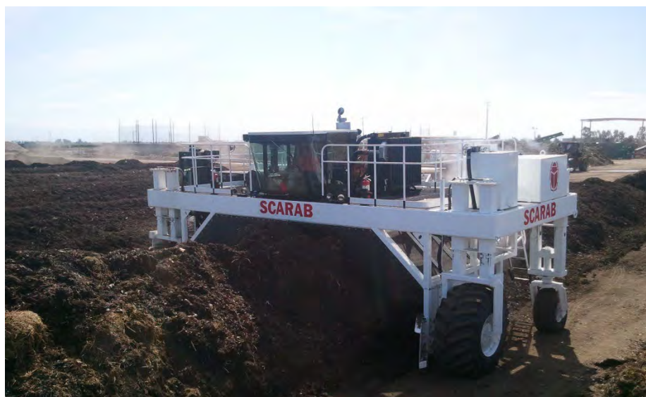
Figure 4. Scarab Model 12 Windrow Turner.
